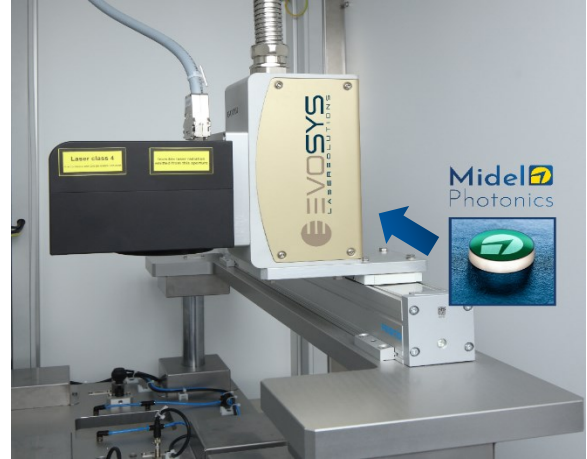
Fig. 3: Optical setup for laser beam joining with integrated Midel Photonics beamshaping optic
