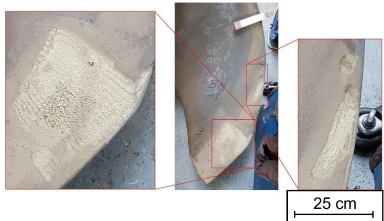
Fig. 1. Cavitation damage to the blade of the ship's propeller (Quelle: LaserCladdingGermany GmbH).
