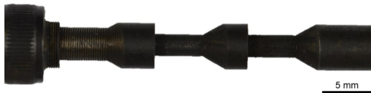
Fig. 4: Initial turning trials. Cut A, B, and C from left to right.
