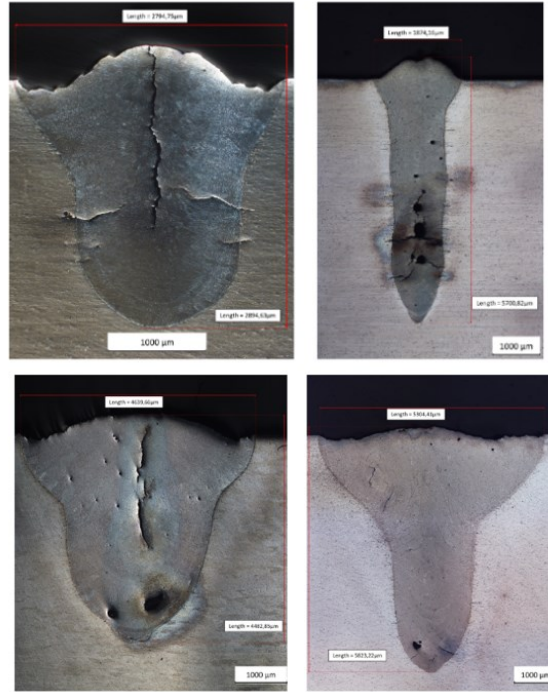
Figure 2: Samples are shown in order as follows: S4 (above left core: 1 kW, ring: 4 kW), S13 (above right, core: 4 kW, ring: 1 kW), S39 (below left core: 1 kW, ring: 4 kW), and S48 (below right, core: 4 kW, ring: 1 kW). Velocity: 100 mm/s (S4 & S13) and 30 mm/s (S39 & S48)
