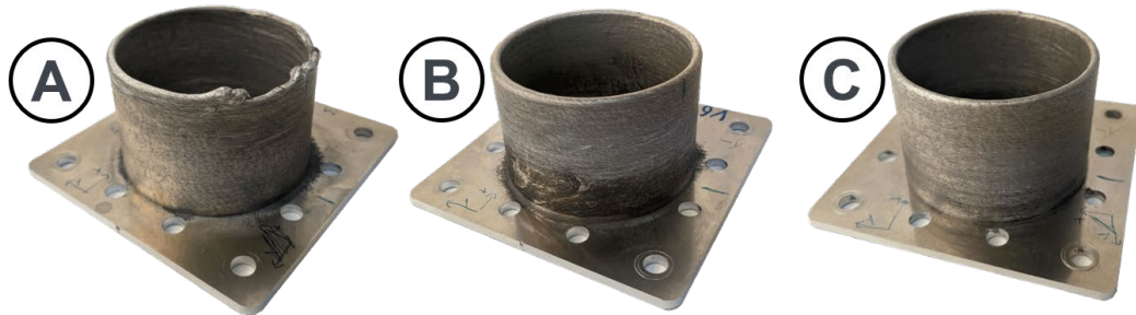
Fig. 3. Result with constant parameters (A), sample produced with variable wire feed rate (B), sample produced with variable wire feed rate and variable irradiated laser power (C).
