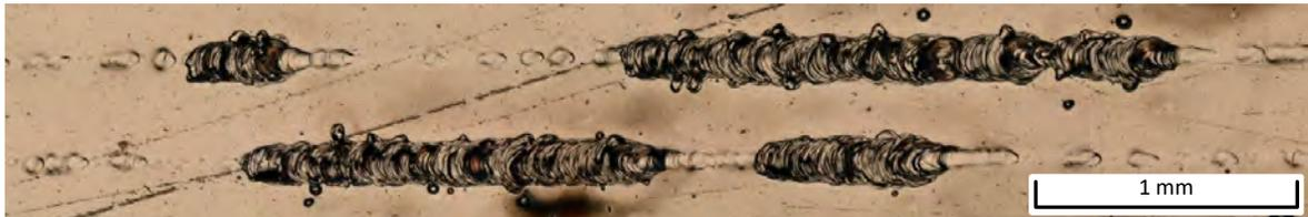
Fig. 16. Interrupted melt tracks due to the high reflectance of the polished copper ETP. Heat conduction and keyhole welding triggered by a large visible scratch.  $P_L = 650$  W,  $v_s = 400$  mm/s,  $d_s = 83$   $\mu$ m.
