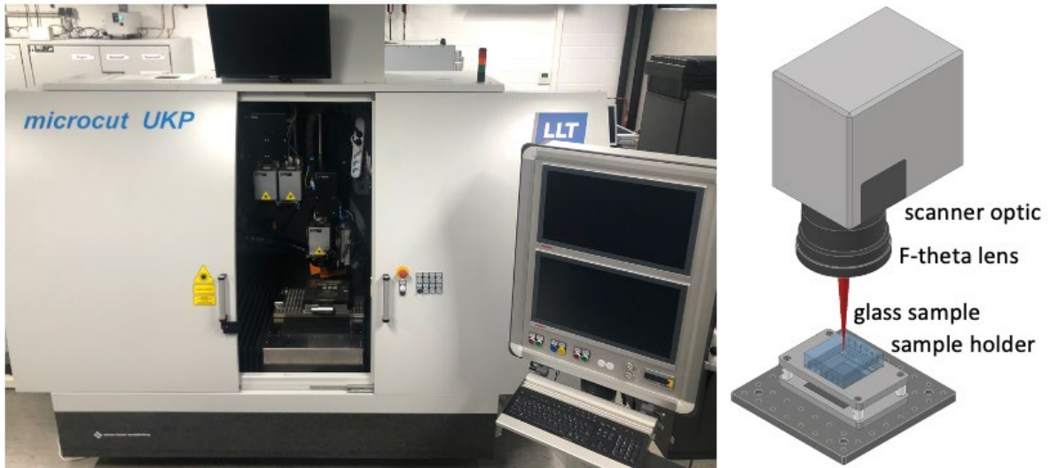
Fig. 1. Experimental set-up for the waveguide inscription and LLT microcut UKP system
