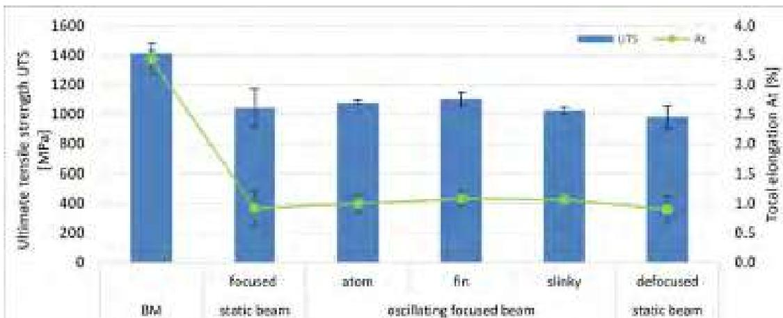
Fig. 6. Tensile characteristics of base metal and laser welds (error bars represent the standard deviation)
