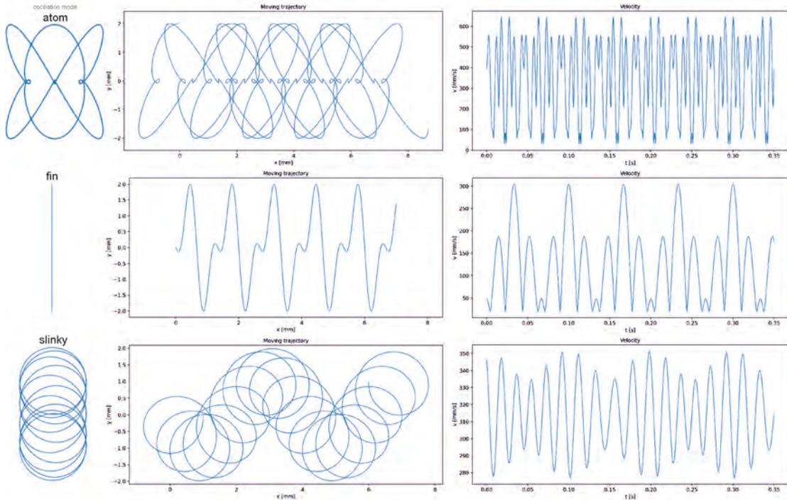
Fig. 1. Applied oscillation modes, corresponding beam trajectories, and spot speed on the material surface
