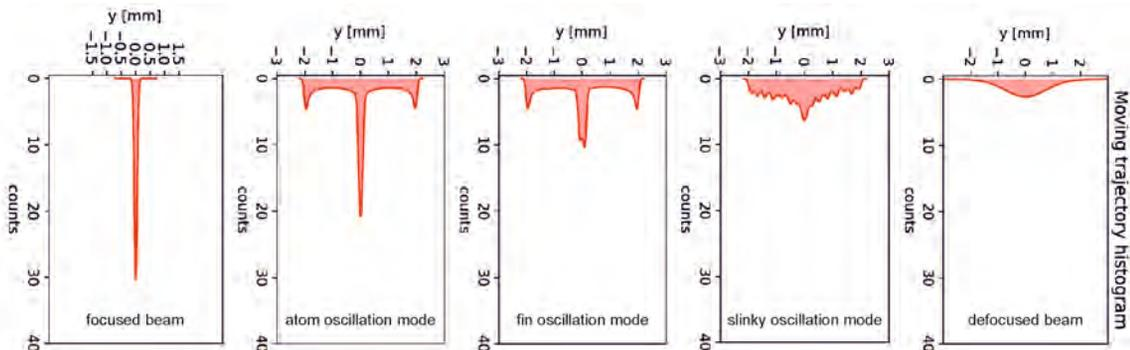
Fig. 2. Histograms of laser spot trajectory for individual welds
