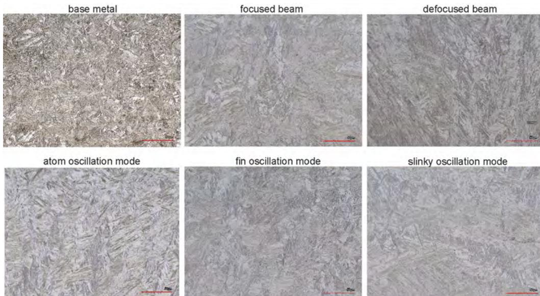
Fig. 4. Base metal and weld metal microstructure, scale 50  $\mu$ m
