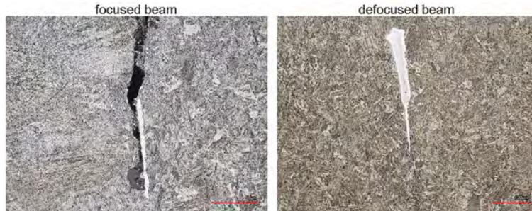
Fig. 5. Defects present on the fusion line of the weld made with the focused beam (scale 50  $\mu\text{m}$ ) and in the WM of the weld made with the defocused beam (scale 100  $\mu\text{m}$ ).
