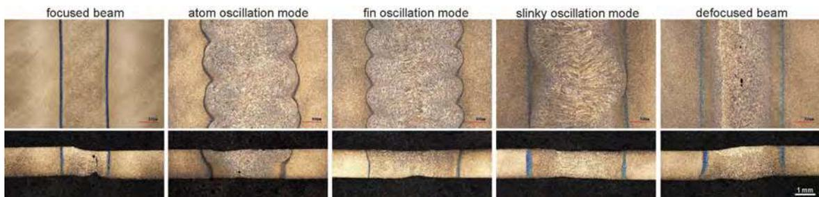
Fig. 3. The surfaces (upper) and the cross-sections (lower) of individual welds
