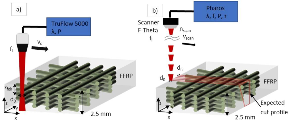
Fig. 2. Experimental setup for cw-laser cut in a) and USP-laser cut in b)
