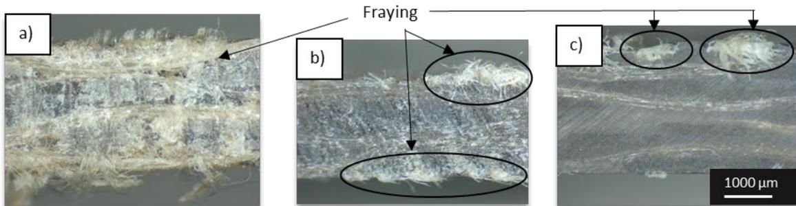
Fig. 1. Examples of mechanical cutting of FFRP with different tools: a) hand saw, b) milling machine, c) wet saw
