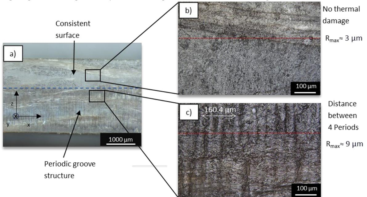
Fig. 4. USP- cut surface at 30x Magnification a); 400 x Magnification of homogeneous region b); 200 x magnification of periodic groove structure ; USP process parameters:  $\lambda = 1030 \text{ nm}$ ,  $P = 12 \text{ W}$ ,  $f = 50 \text{ kHz}$ ,  $\tau = 250 \text{ fs}$ ,  $v_s = 120 \text{ m/min}$ ,  $M^2 = 1.2$ ,  $d_0 = 57 \mu\text{m}$ ,  $d_h = 50 \mu\text{m}$ ,  $N_s = 3750$ ,  $Z_{\text{fok}} = 0 \text{ mm}$ ;
