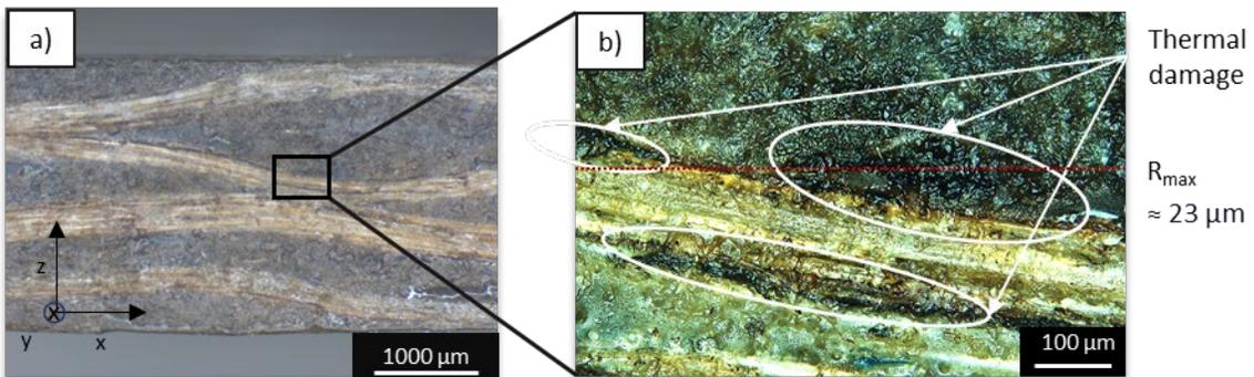
Fig. 3. cw-cut surface at 30x magnification in a) and 200x Magnification in b); cw process parameters:  $\lambda = 10.6 \mu\text{m}$ ,  $P = 700 \text{ W}$ ,  $v_c = 8 \text{ m/min}$ ,  $M^2 = 2.3$ ,  $d_o = 230 \mu\text{m}$ ,  $z_{\text{fok}} = -0.5 \text{ mm}$
