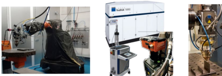
Fig. 1. Robotic laser metal deposition workstation and process and control equipment of the experimental setup
