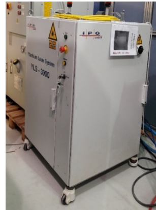
Fig. 3. IPG YLS 300 fiber laser source
