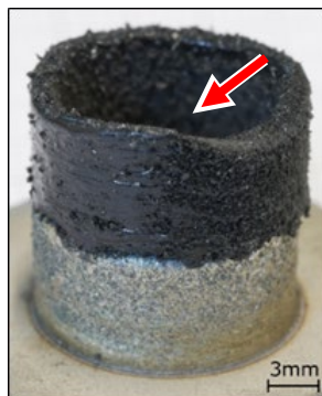
Fig. 5. Hollow cylindrical structure on a further perpetrated stainless steel substrate. Material accumulation is marked.
