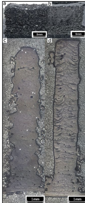
Fig. 4. Multi track wall structures; (a) Surface without remelting; (b) Surface with remelting; (c) Cross-section without remelting; (d) Cross-section with remelting.
