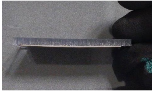
Fig. 6. Hybrid polymer-metal joint after 400 thermal shock cycles
