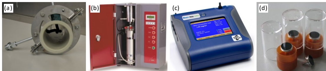
Fig. 2. Selection of sampling systems used (cf. Walter et al., 2019); (a) pipe with manifold for isokinetic sampling, e.g. on TruPrint systems; (b) ELPI™ (low pressure electrical cascade impactor → particle size distributions); (c) TSI DustTrak™ DRX (analysis of light scattering → 4 different particle fractions); (d) pin stub holder (capture of redeposits) → SEM/EDX, chemical analysis).
