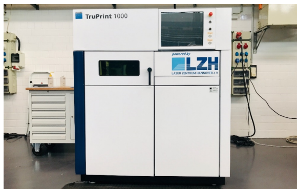
Fig. 1. LPBF system TruPrint 1000 of Trumpf Laser- und Systemtechnik GmbH used for the LPBF process simulated at the LZH.
