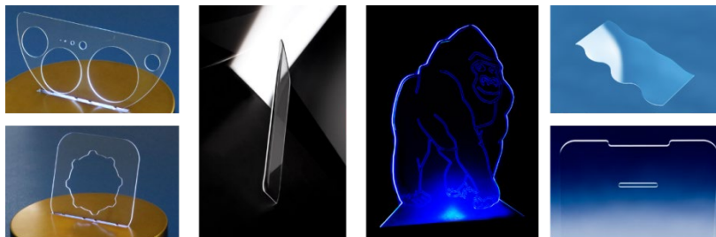
Fig. 3. Inner (1 st column) and outer (3 rd & 4 th column) contours generated with the Corning® glass cutting technology. The second column presents a 3D part cut by Corning® glass cutting technology.
