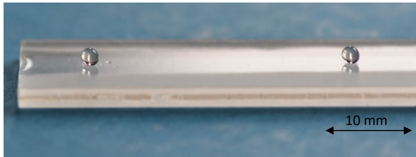
Fig. 3. Glass spheres with a diameter of 2 mm melted together from fragments of the supplied fiber as a result of an too high energy input of 135 W.
