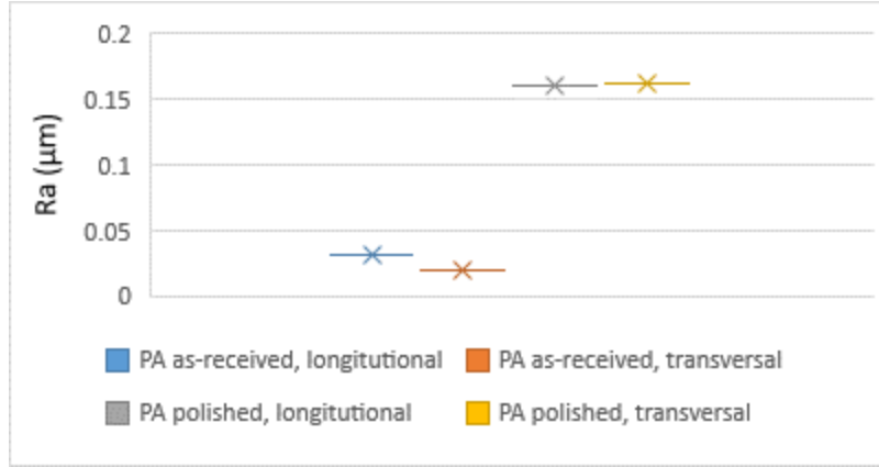
Fig. 10. Roughness measurement of the PA surface.
