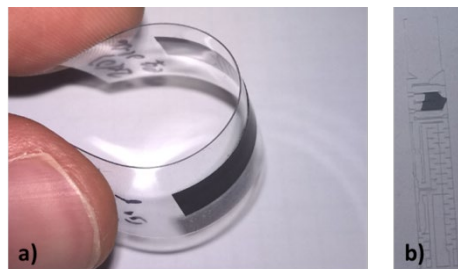
Fig. 5. (a) Bending test of mock-up welding circuit; (b) remains on transparent foil after peel-off test of mock-up welded circuit
