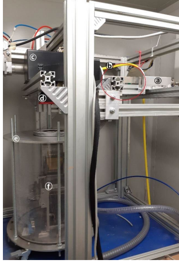
Fig.3. The integrated SLM system. (a) Remote amplifier of the laser source, (b) collimating unit, (c) scanner head, (d) f-theta lens, (e) protective window, (f) powder-bed.
