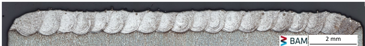
Fig. 3. Microsection of buttering
