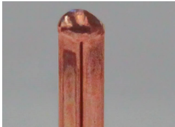
Fig. 19. Hairpins welded with the 500-Watt blue laser with no porosity or spatter.
