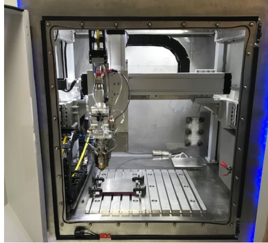
Fig. 4. Gantry system used for testing the welding characteristics of the blue laser system and BlueWeld™ processing head.
