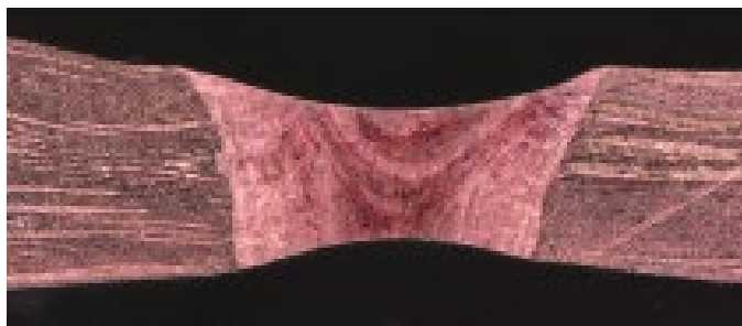
Fig. 15. Stack of 40 – 10 \mu\text{m} foils welded with the 500-Watt laser.
