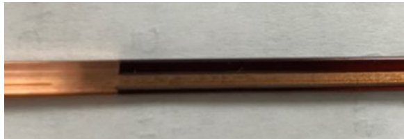
Fig. 18. Stripping of the insulation on a 1.5 mm x 4 mm copper conductor using 150 Watts at 6 m/min.
