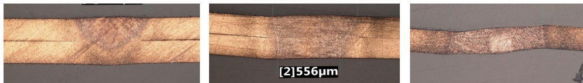
Fig. 9. Lap welds of 2 sheets of 200 \mu\text{m} thick copper, at 500W and 230 \mu\text{m} beam diameter. (left) partial penetration; (center) full penetration. (right) butt weld of the same sheets.
