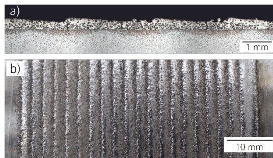
Fig. 3. a) Cross section of a single layer coating of NiCrBSi+60%WC on mild steel type S235, manufactured by HPLC. b) Top view of a single-layer coating of NiCrBSi+60%WC on mild steel type S235 with 20 tracks next to each other on a pipe section, manufactured using HPLC.
