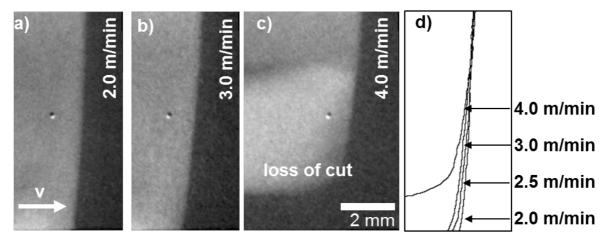
Fig. 3. Average images from X-ray videos for different feed rates (a-c). Extracted geometries of the cutting front for different feed rates (d).
