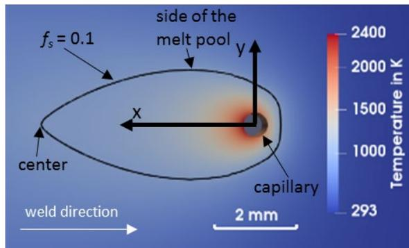
Fig. 2. Resulting temperature field for a simulation of the aluminum alloy AA6016 with  $P = 3.3$  kW,  $v = 3$  m/min,  $s = 2.4$  mm,  $d_f = 600$   $\mu$ m,  $\eta = 0.83$ . The black line indicates the contour with  $f_s = 0.9$ .
