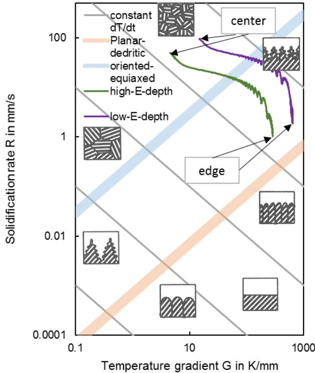
Fig. 4. Solidification structure map according to Kurz and Fisher, 1992 with the simulated results. With  $P = 0.8$  kW,  $v = 6$  m/min,  $d_f = 100$   $\mu$ m,  $s = 1.2$  mm (low- $E_{depth}$ ) and  $P = 3.3$  kW,  $v = 3$  m/min,  $d_f = 600$   $\mu$ m,  $s = 2.4$  mm (high- $E_{depth}$ ). Valid for a solidification interval  $\Delta T \approx 50$  K.
