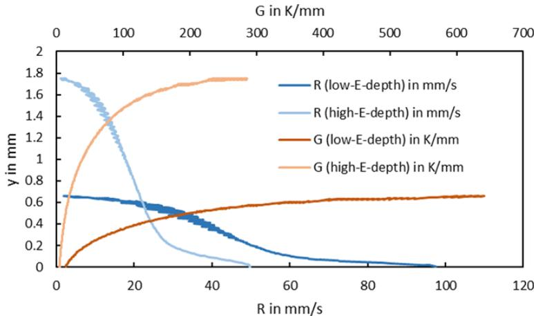
Fig. 3. Numerically calculated values of the temperature gradient  $G$  and the solidification rate  $R$  at the respective  $y$ -coordinates for  $f_s = 0.9$ . With  $P = 0.8$  kW,  $v = 6$  m/min,  $d_f = 100$   $\mu\text{m}$ ,  $s = 1.2$  mm (low- $E_{depth}$ ) and  $P = 3.3$  kW,  $v = 3$  m/min,  $d_f = 600$   $\mu\text{m}$ ,  $s = 2.4$  mm (high- $E_{depth}$ ).
