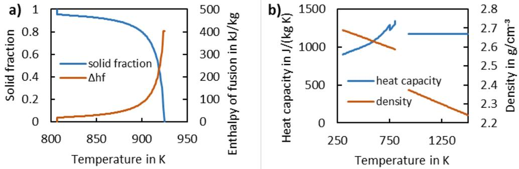
Fig. 1. Temperature dependent properties calculated with *Thermo-Calc 2018a TCAL5 Al-Alloys database version 5.1*, as shown in Andersson et al., 2002. (a) Temperature dependent solid fraction  $f_s$  and integral of enthalpy of fusion. (b) Calculated temperature dependent values of heat capacity and density.
