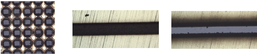
Fig. 12. Invar square and trenches processing (a) 1 pass; (b) 10 passes; (c) 100 passes
