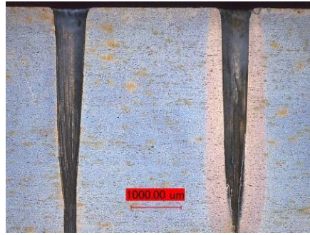
Fig. 3. The effect of heat accumulation on drilling with a pulse energy of 2 mJ and a repetition rate of 60 kHz (left hole) and 100 kHz (right hole). The orange colour indicates the heat affected zone which is revealed after etching of the cross section.
