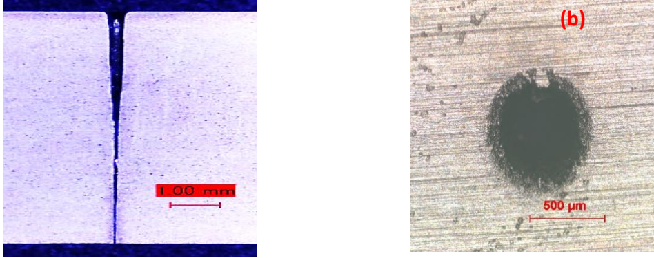
Fig. 4. The drilling depths of 8.0 mm achieved with the pulse energies of 1.3 mJ in the repetition rate of f_R = 30 kHz (a), the inlet quality (b). No phase transition is observed in the depth and on the surface.
