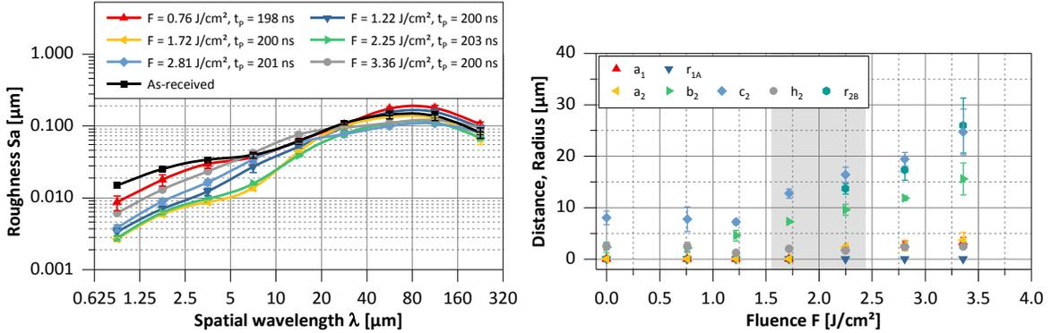
Fig. 3. (a) Roughness spectra of the surfaces laser micro polished with the laser beam source redENERGY G3 and different fluence; (b) Distances and radii of the corresponding edges in dependence on the fluence
