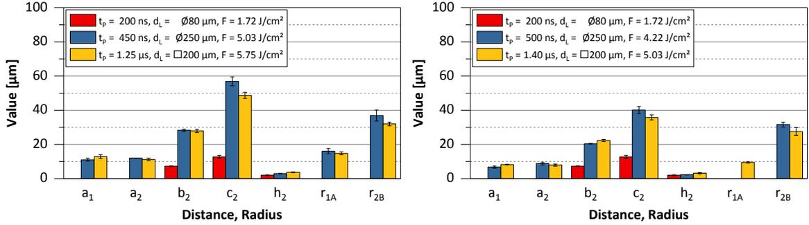
Fig. 4. (a) Distances and radii of the edges of the surfaces with the lowest roughness achieved for the three different pulse duration regimes
