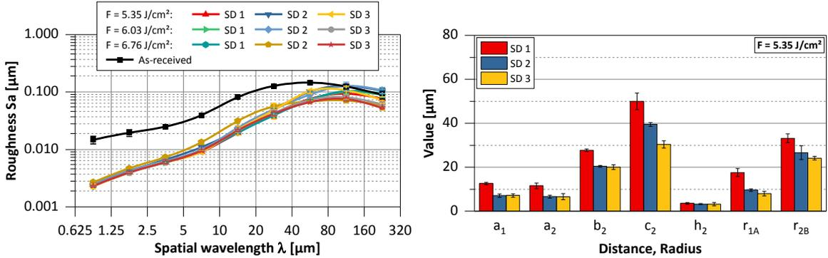
Fig. 5. (a) Roughness spectra of the surfaces laser micro polished with different scanning direction and fluence (TruMicro 7050); (b) Distances and radii of the edges polished with a fluence of  $F = 5.35 \text{ J/cm}^2$  and different scanning directions
