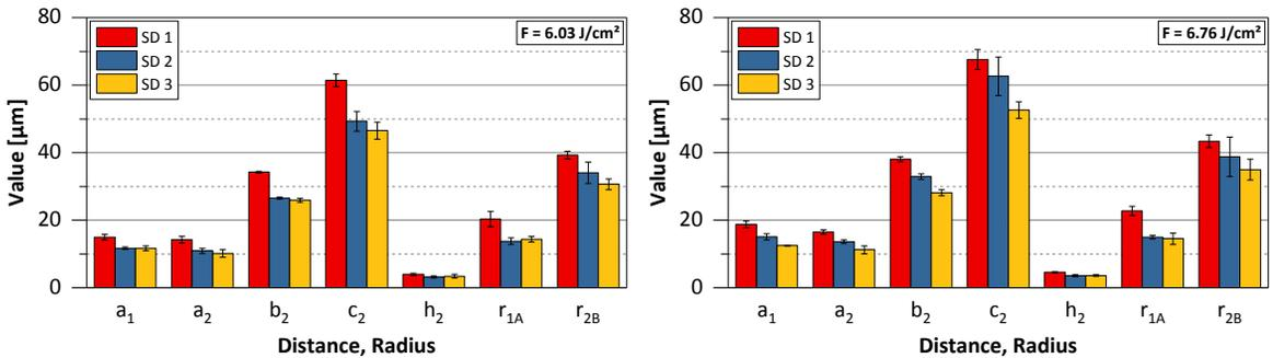
Fig. 8. Distances and radii of the edges polished with the laser beam source TruMicro 7050, a fluence of (a)  $F = 6.03 \text{ J/cm}^2$ , (b)  $F = 6.76 \text{ J/cm}^2$  and different scanning directions
