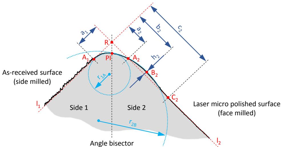
Fig. 1. Profile of laser micro polished edge with measured distances and radii
