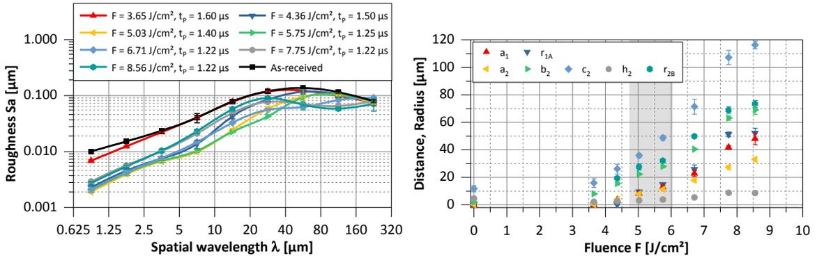
Fig. 7. (a) Roughness spectra of the surfaces laser micro polished with the laser beam source TruMicro 7050 and different fluence; (b) Distances and radii of the corresponding edges in dependence on the fluence
