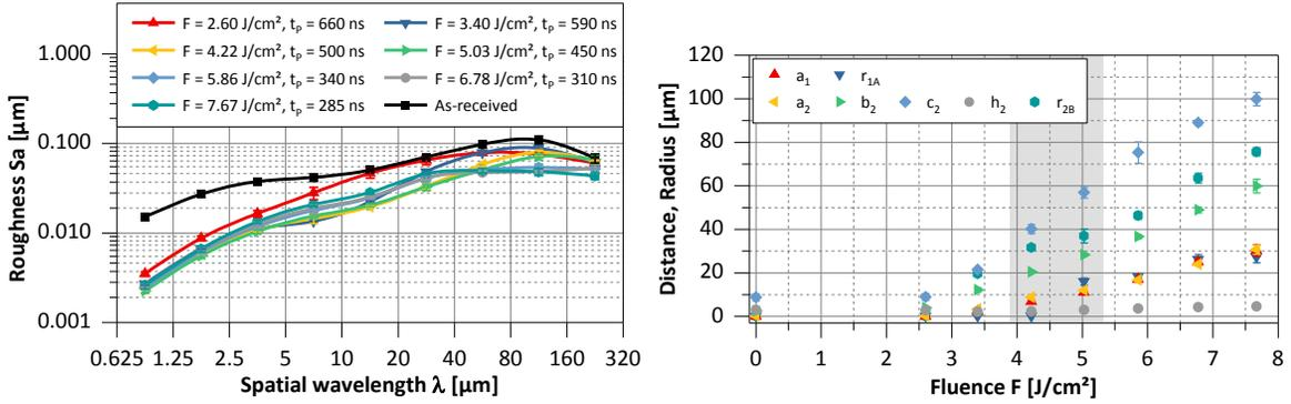
Fig. 6. (a) Roughness spectra of the surfaces laser micro polished with the laser beam source HPQL and different fluence; (b) Distances and radii of the corresponding edges in dependence on the fluence
