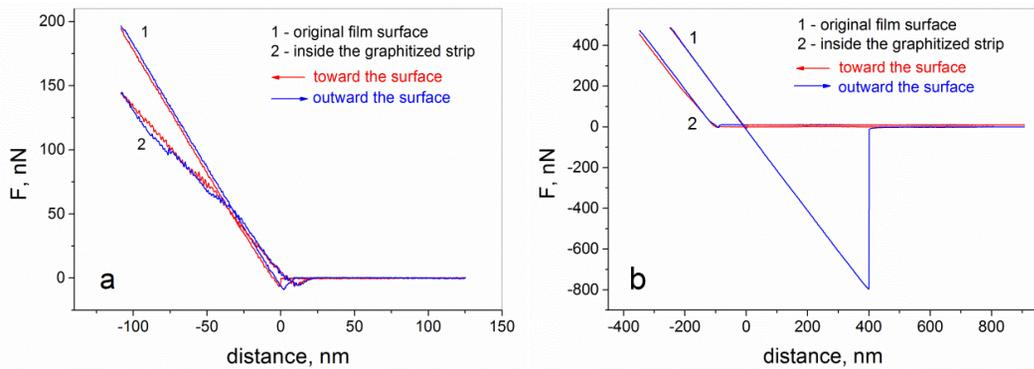
Fig. 5. Force-distance curves for the contacts of the sharp (a) and blunt (b) Si tips inside and outside the laser-graphitized strip (shown in Fig. 4); the curves 2 in (b) are shifted by 100 nm along the X axis for clarity.
