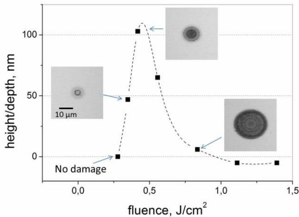
Fig. 1. Height/depth in the center of laser spots vs peak fluence during single-pulse irradiation of the DLN film (along with OM images of several spots); no damage is observed at the fluence  $E=0.28$  J/cm<sup>2</sup>.
