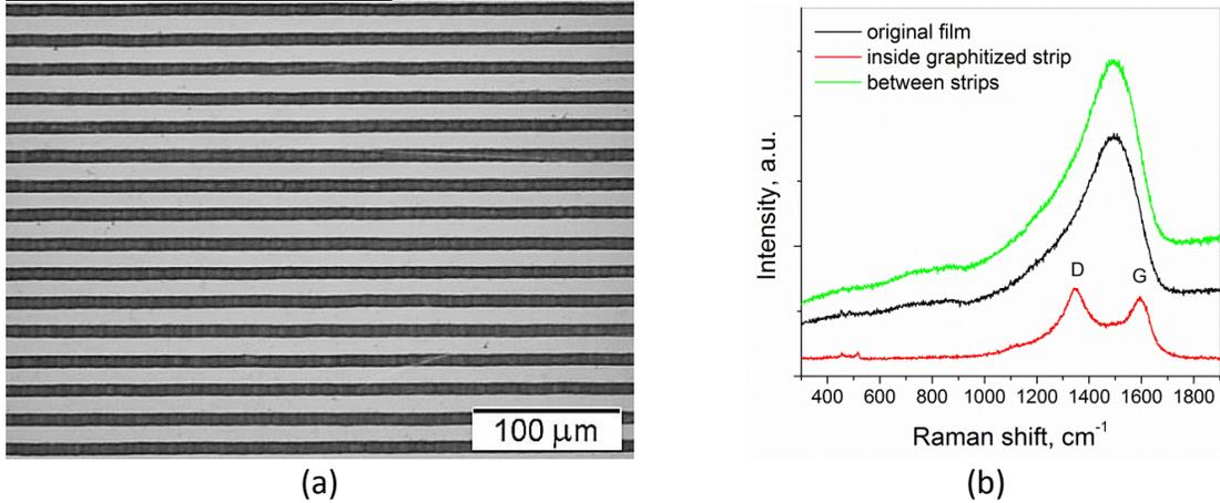
Fig. 3. (a) Periodic linear micropattern (graphitized strips of  $<10 \mu\text{m}$  width and  $20 \mu\text{m}$  period) fabricated on the DLN film surface during fs-laser multipulse irradiation at the pulse energy  $\epsilon=2 \mu\text{J}$  (peak fluence  $E=0.28 \text{ J/cm}^2$ ), and scanning beam velocity  $0.05 \text{ m/s}$ . (b) Raman spectra of the original film and laser-patterned region (inside the laser-irradiated strips and between the strips).
