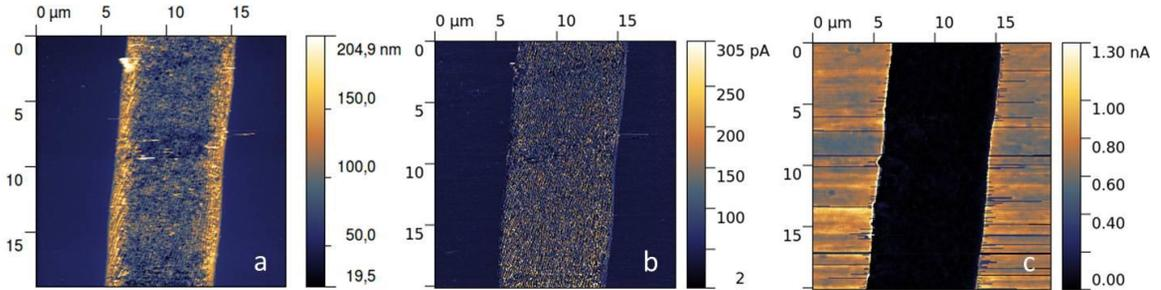
Fig. 4. Surface relief (a) and friction force (b,c) images of the laser-graphitized strip recorded with a sharp Si tip of  $R_{tip} = 10$  nm at load on the tip  $F = 24$  nN (a,b) and with a blunt Si tip of  $R_{tip} = 1.5 \mu\text{m}$  at load  $F = 6$  nN (c); the scale in friction images is given in the deflection angle of the cantilever [Zavedeev et al., 2017].
