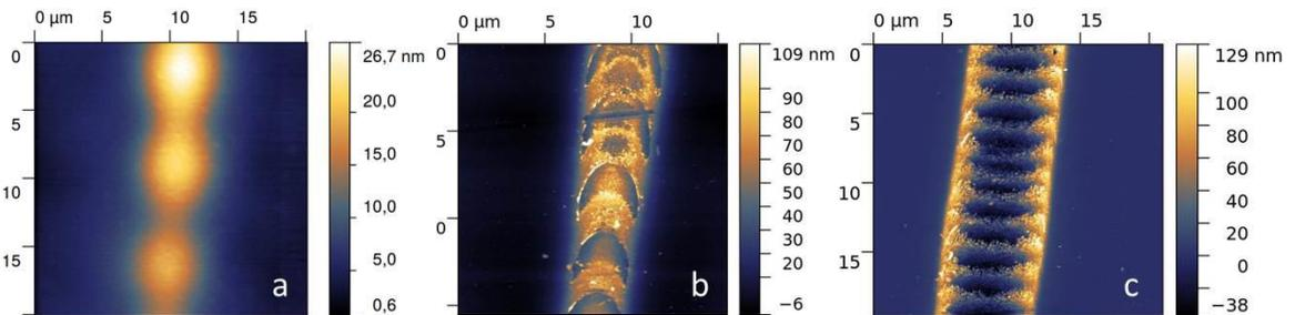
Fig. 2. AFM images of laser-irradiated regions formed during multipulse irradiation at the pulse energy  $\epsilon=2 \mu\text{J}$  (fluence  $E=0.28 \text{ J/cm}^2$ ) and different scanning beam velocities: (a)  $0.8 \text{ m/s}$ , (b)  $0.4 \text{ m/s}$ , and (c)  $0.2 \text{ m/s}$ .
