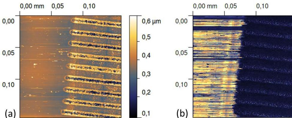
Fig. 6. Surface relief (a) and friction force (b) images (recorded with a blunt Si tip of  $R_{tip}=1.5 \mu\text{m}$  at load  $F=64$  nN) of the periodic linear micropattern fabricated on the DLN film surface during multipulse irradiation at the pulse energy  $\epsilon=2 \mu\text{J}$  (fluence  $E=0.28 \text{ J/cm}^2$ ) and scanning beam velocity 0.05 m/s.
