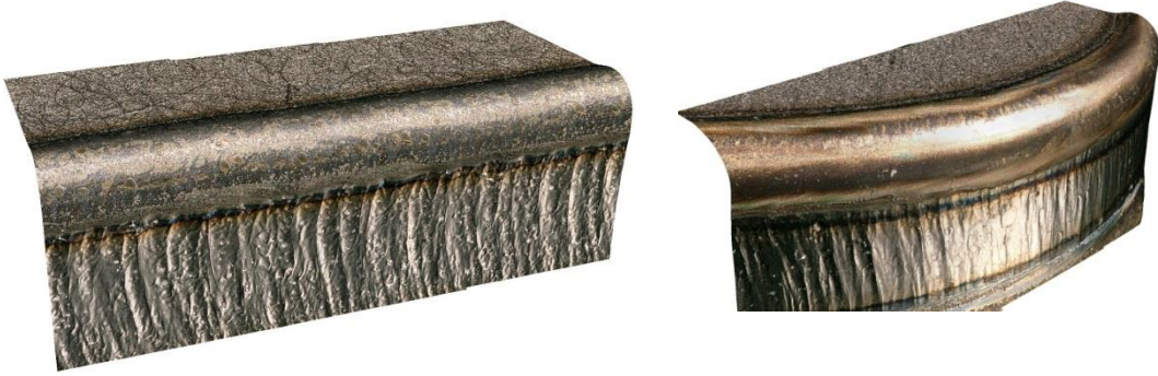
Fig. 6. (a) 3D image of a deburred linear edge (parameter setting 2, position: middle); (b) 3D image of a deburred round edge (parameter setting 2)
