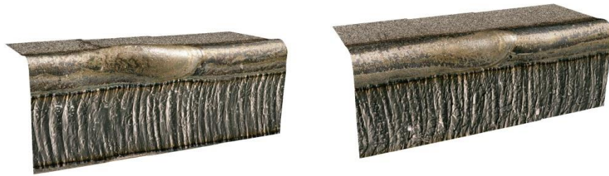
Fig. 10. (a) 3D image of a SLD transition (parameter setting 2, strategy 2); (b) 3D image of a SLD transition (parameter setting 2, strategy 3);
