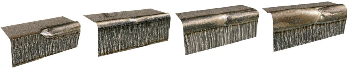
Fig. 9. (a) 3D image of the end of a deburred edge (parameter setting 2); (b) 3D image of a SLD transition (parameter setting 1, strategy 1); (c) 3D image of a SLD transition (parameter setting 2, strategy 1); (d) 3D image of a SLD transition (parameter setting 2, strategy 1)
