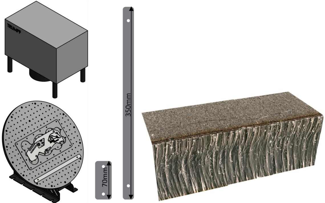
Fig. 3. (a) Experimental setup; (b) Samples; (c) Digital 3D image of an edge geometry before deburring (Keyence VHX-5000)
