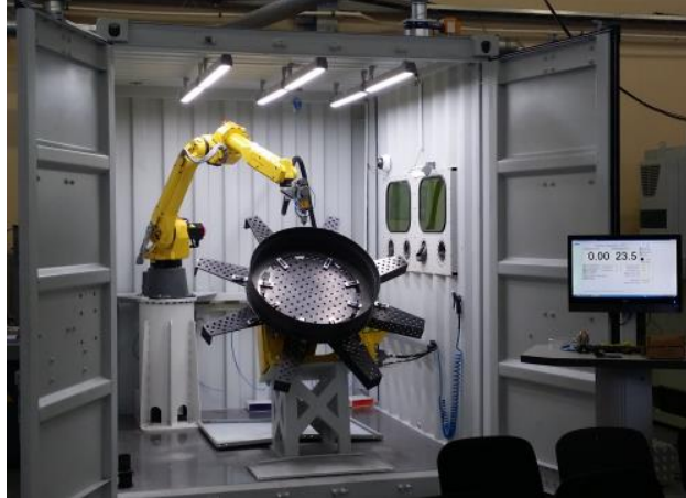
Fig. 3. Direct laser metal deposition machine, size “XL”.
