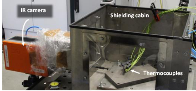
Fig. 6. Experimental set-up for empirical validation of numerical heat input
