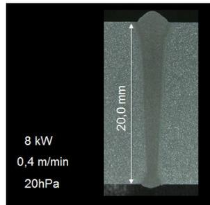
Fig. 10. Micrograph through weld, MoVac, 20 hPa
