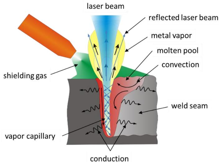
Fig. 2. Joining zone in laser beam deep welding
