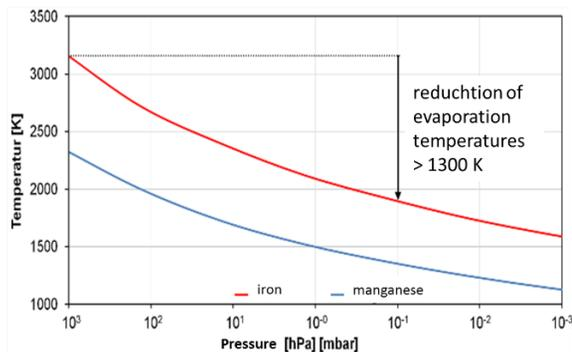
Fig. 4. Vapor pressure curve of iron, manganese
