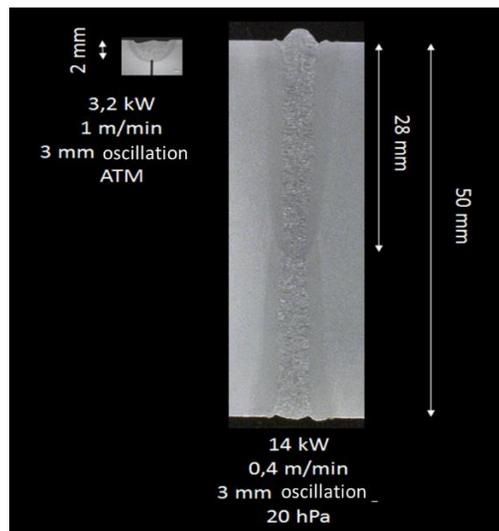
Fig. 11. Micrograph sealing weld (left) and joining weld (right), MoVac, 20 hPa
