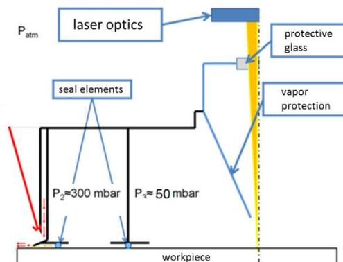
Fig. 8. Schematic setup of the mobile vacuum chamber
