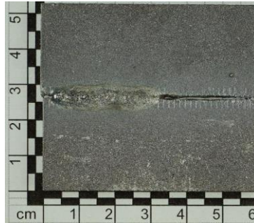
Fig. 14. Welding of support – support: surface of weld (no cross section possible)
