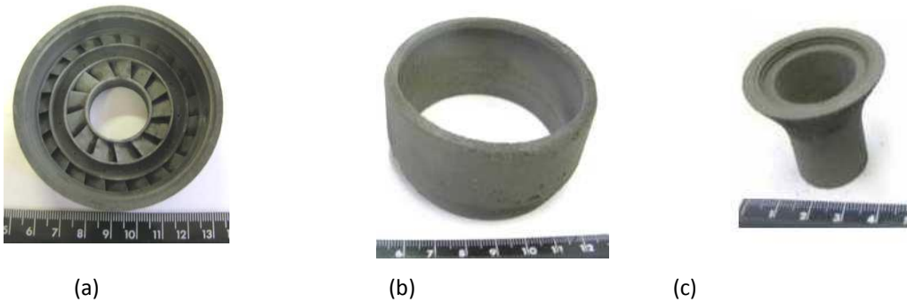
Fig. 6. Ceramic combustion chamber with uncooled flue pipes and cleaner burning of fuel in the counter-offset swirling jets for multimodular gas turbine engines power up to 32 MW: front device – (a), external flame tube – (b), internal flame tube – (c).
