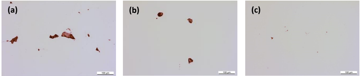
Fig. 1. Representative microstructures with pores for the quality levels: (a) poor quality; (b) medium quality and (c) high quality
