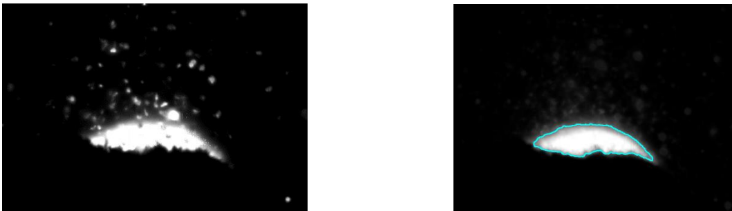
Fig. 2. (a) gray scale image of the melt pool; (b) segmentation of the melt pool
