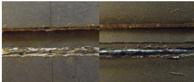
Fig. 6. Fracture surfaces of lap shear tests with (l) and without (r) coating
