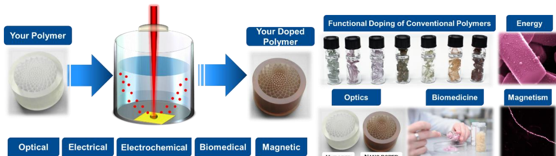
Fig. 2: Scheme of direct polymer doping by pulsed laser ablation in liquid monomer or polymer solution with ligand-free nanoparticles (left, structures manufactured by microTEC) and different application options (right)
