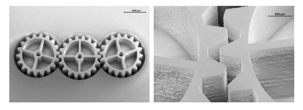
Fig. 2: Overview on micro machined soda lime glass
