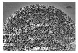
Fig. 4: Overview of drilled structures in 1000  $\mu m$  thick soda lime glass
