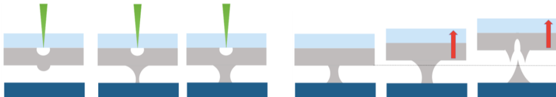
Figure 3. Scheme of the LIFT process for high viscosity pastes. Left: Column generation. Right: Glass removal and final shape definition.
