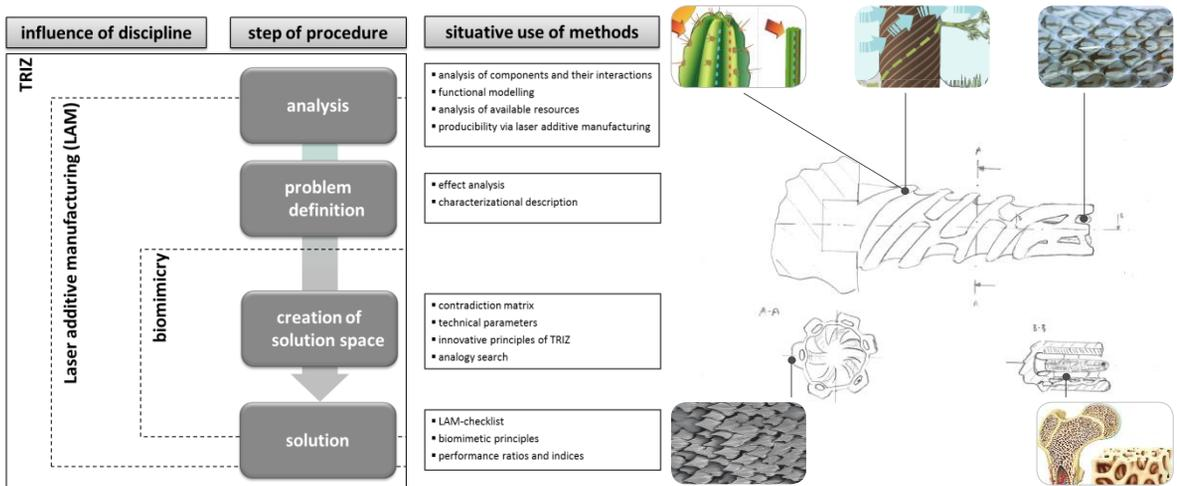
Fig. 2. Left: schematic view of the introduced TRIZ-based methodology for biomimetic part optimization for LAM, right: preliminary sketch of the reamer as a combination of technical feasible biomimetic analogies for part optimization specifically for LAM
