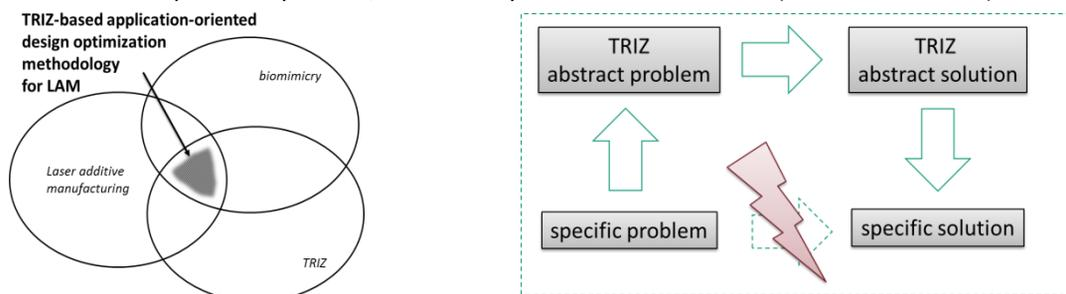
Fig. 1:left: schematic view of the considered disciplines focused for development of an application-oriented design optimization TRIZ-based methodology for LAM; right: general problem solving approach used in TRIZ
