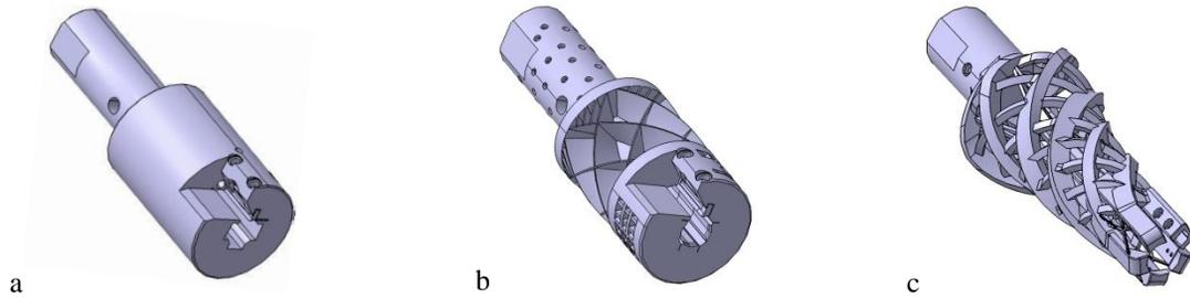
Fig. 4. Evolutionary development of the case study external reamer: (a) original reamer; (b) design of a practitioner without methodological support; (c) result of a systematic design for LAM using augmented TRIZ, (a) and (b) is the result of a topology optimization conducted together with MAPAL Dr. Kress KG (Schneider 2013)
