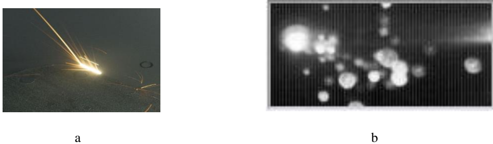
Fig. 1 Images of SLM process in visible (a) and infrared (b); integral (a) , (b) high-speed shooting ( Smurov , 2009)
