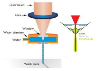
Fig. 1. Schematic of the water jet guided laser.
