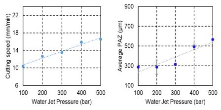
Fig. 2. Effect of water jet pressure on cutting performance.
