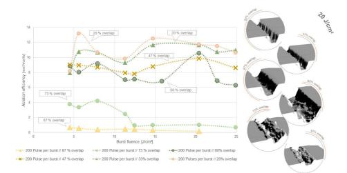
Fig. 2. Line scribing obtained with 515 nm GHz bursts on silicon. The effect of the pulse overlap is shown both on the ablation efficiency and on the scribing quality.
