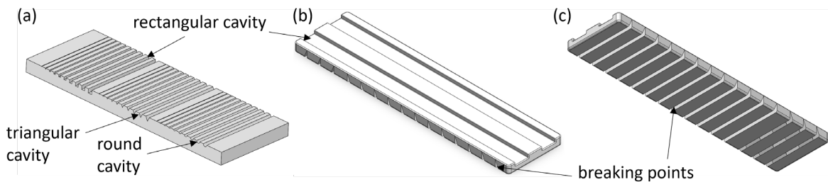
Fig. 4. (a) Substrate with cavities in various shapes and dimensions; (b) Substrate with cavities and fractures (top view); (c) Substrate with cavities and fractures (backside)
