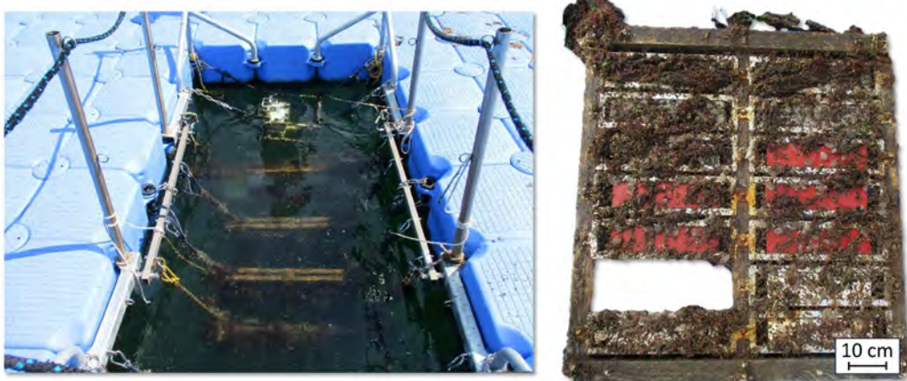
Fig. 2. Left - Swimming pontoon in the North Sea with a hole inside where sample racks can be stored underwater. Right - biofouling samples in the sample frame after an immersion period of several weeks.
