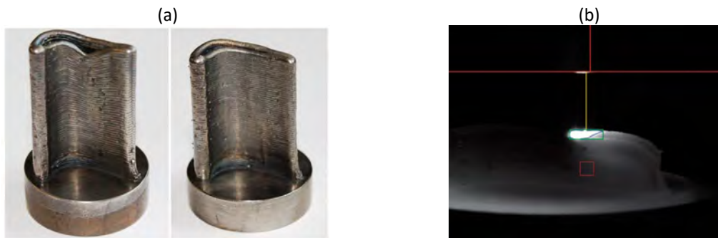
Fig. 5. (a) Deposited CM 247 LC on Inconel 718 substrate material as a near net shape blade geometry. The substrate was preheated to 1100 °C to obtain a reduction of defects, (b) etched cross section at position A, (c) etched cross section at position B, all images adapted from [23]
