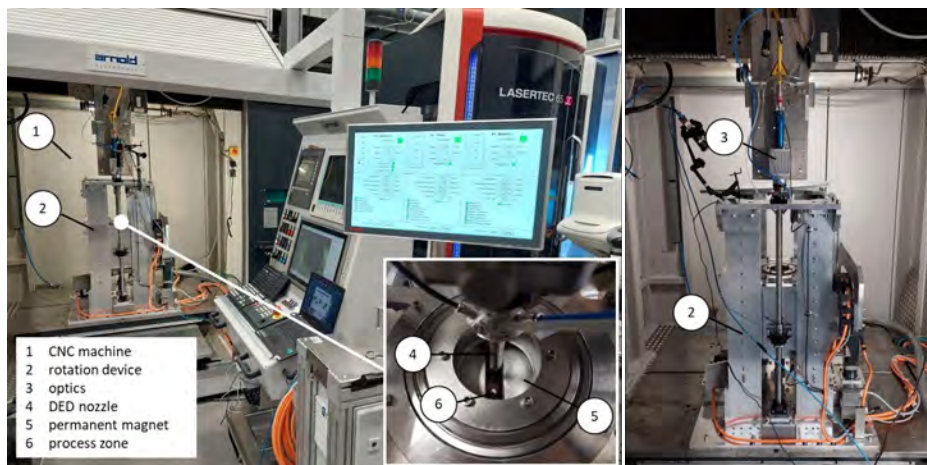
Fig. 2. Experimental set up for the investigation of the influence of static and rotating electromagnetic fields on the solidification microstructure and crack formation
