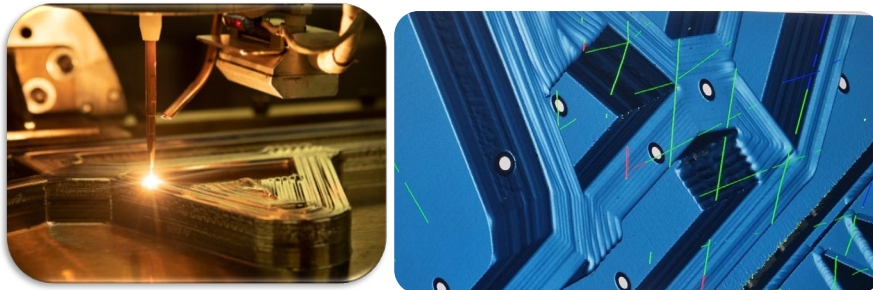
Fig. 6. (a) Manufacturing of the near net shape for the flap track demonstrator by W-DED-LB process; (b) Dimensional control by 3D scanning.
