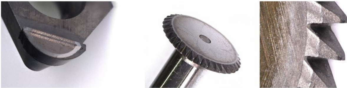
Fig. 12. A cutting tool edge (left) and a diamond cutting wheel (middle and right) as-processed.
