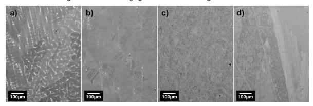
Fig. 1. SEM micrographs displaying a longitudinal section of each fabrication technique: (a) casting; (b) milling from disk; (c) SLM; and (d) LDED.
