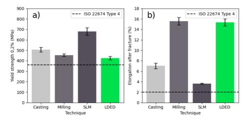
Fig. 2. Yield strength 0,2% (a) and Elongation after fracture; (b) of all materials obtained by casting, milling from disk, SLM and LDED.
